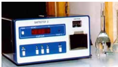
Fig. 1. Toxicity tester, biotester-2 concentration meter
